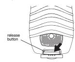
3 Allow the battery door to pop up, slide it forward, and remove it from the back of your phone.
